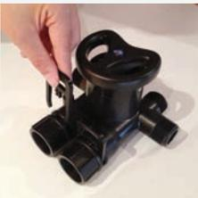
Remove the clips on the threads.
