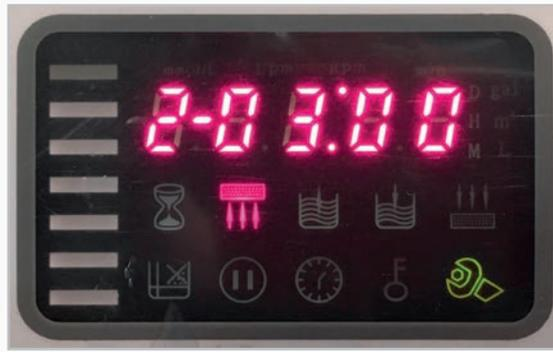
With the help of the UP and DOWN keys, indicate the duration of the back-up of your water softener (Table 2 shows the corresponding value for each model). Press "menu / confirmation" to confirm.
