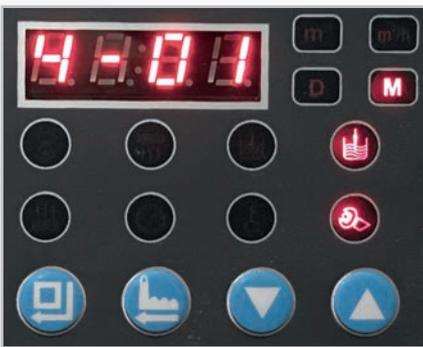
Using the "menu / confirmation" key, and with the help of the UP and DOWN keys, mark the brine charge time of your water softener (table 2). Press "menu / confirmation" to confirm.
