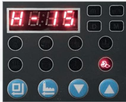
Press "Menu/confirm" and use UP and DOWN to set the number of days you wish, between 00 and 40. That is preset at 30 days. Press "Menu/confirm" to confirm.
