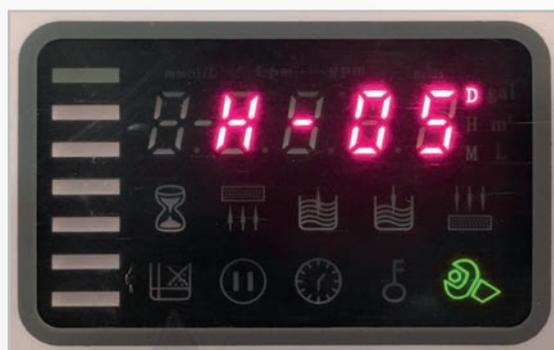
Press "Menu/confirm" and use UP and DOWN to set the number of days you wish, between 00 and 40. That is preset at 30 days. Press "Menu/confirm" to confirm.
