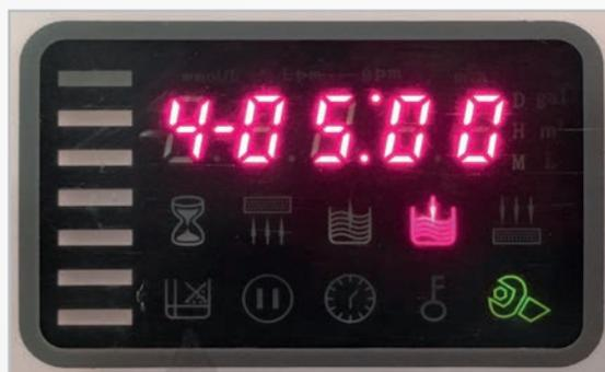
Using the "menu / confirmation" key, and with the help of the UP and DOWN keys, mark the brine charge time of your water softener (table 2). Press "menu / confirmation" to confirm.
