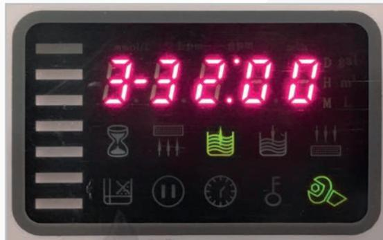
With the help of the UP and DOWN keys, indicate the brine suction time of your water softener (table 2). Press "menu / confirmation" to confirm.
